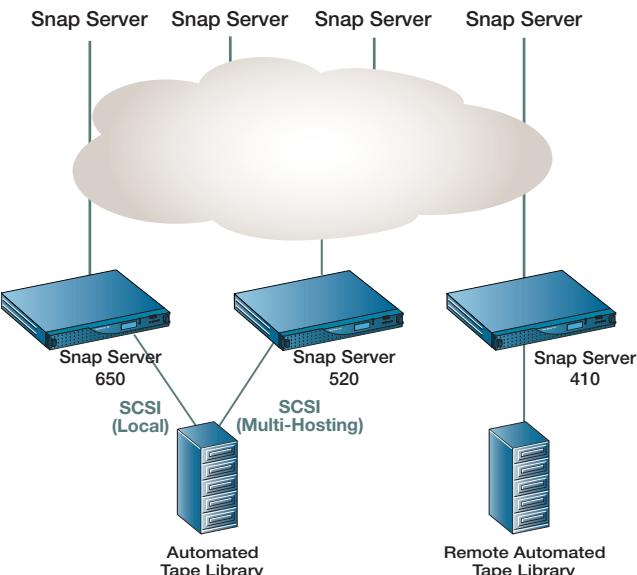
A well-designed, distributed architecture gives BakBone NetVault for GuardianOS the flexibility to exploit advanced data management technologies, including Network Attached Storage (NAS). Some possible topology configurations:
