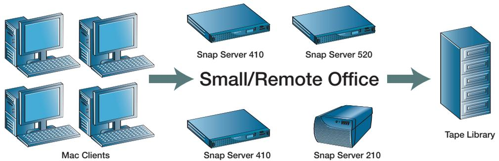
Files from desktops and laptops connected to the network are automatically saved to a Snap Server. No user action or intervention is required.
